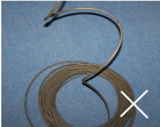
Incorrect method of de-coiling
