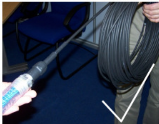
Correct method of de-coiling
